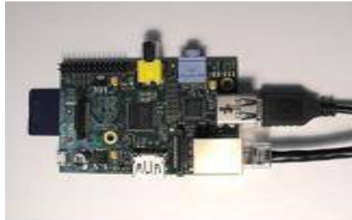
Figure 5: HDMI Cable plugging
