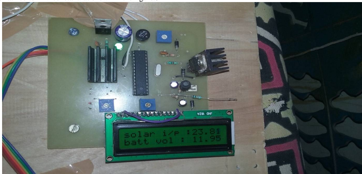
Fig.3 Final stage of solar tracking system.
