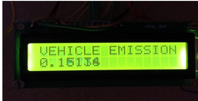
Fig.14: Smoke sensor readings displayed on LCD
