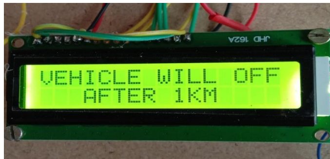
Fig.16: Final Warning Message on LCD Screen
