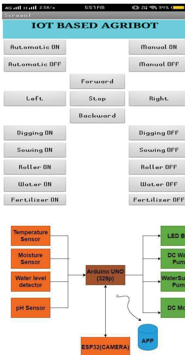
fig. 8. Block Diagram of Monitoring System
