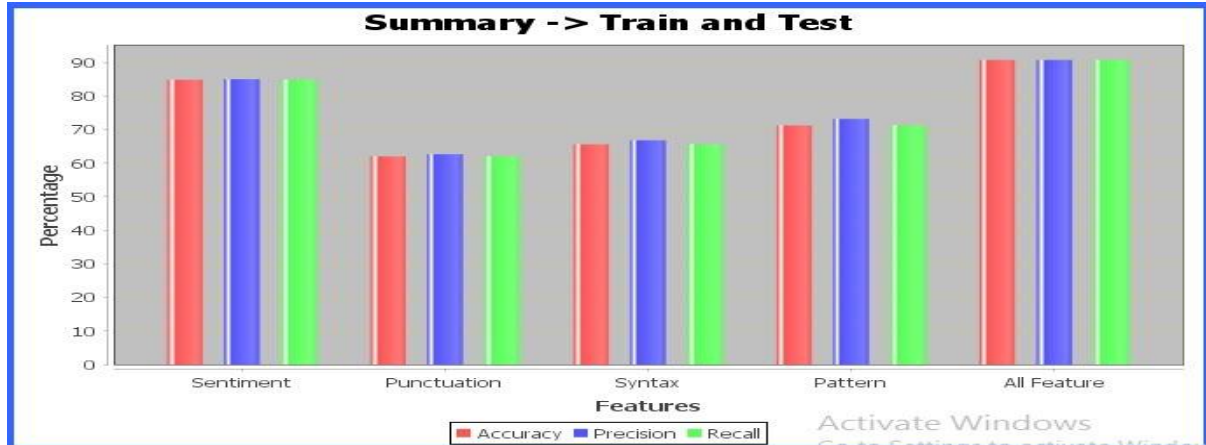
Fig. 3: Accuracy, Precision and Recall of classification during "Train and Test" for each set of features.
