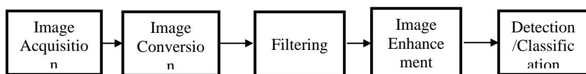
Fig. 1: Basic Steps in Image Processing
