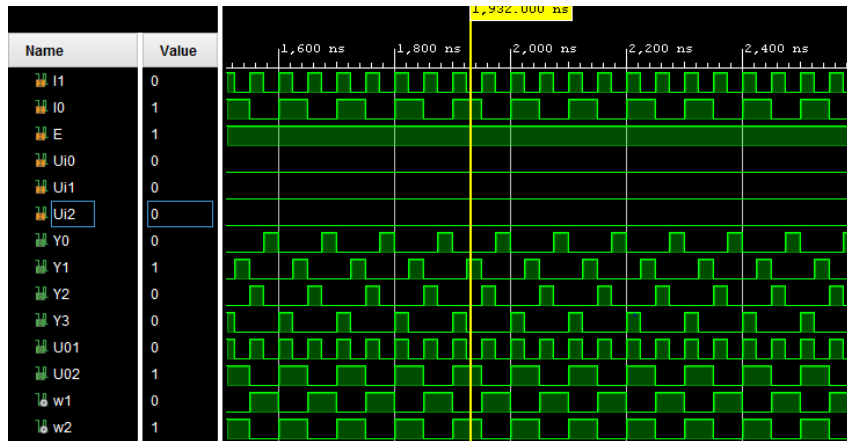
Fig 1.10 : Simulation Waveforms of 2:4 Decoder
