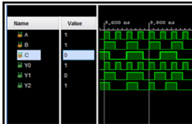
Fig 1.4 : Simulation Waveforms of 2:1 mux
