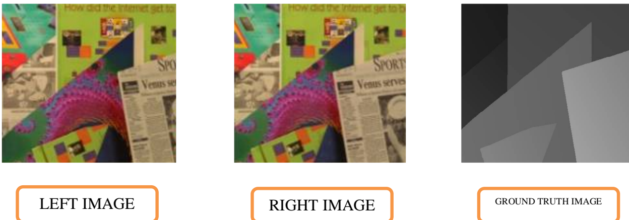
Fig 5: The input left and right images along with its ground tooth image
