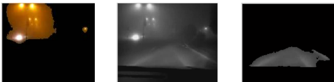
Figure 2: (a) Input Frame 142 and 322; (b) Luminance Image; (c) Binary Image; (d) Segmented Object in Current Frame
