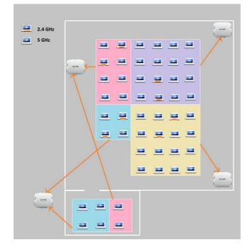
In [B] a dynamic environment of students with proposed methodology, More clients on 5 GHz for better throughput and performance.RF utilization and client to AP signal taken into account when balancing.No more slow clients bringing down the network.High utilization clients are balanced across APs to limit bottlenecks.
