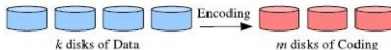
Fig.3: erasure code to encode k disks of data onto m = n - k disks of coding [8]
