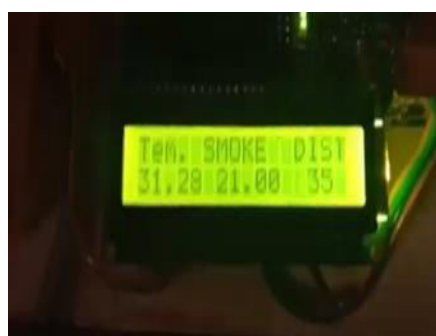
fig 3. The LCD Display shows temperature & smoke value and distance of the object
