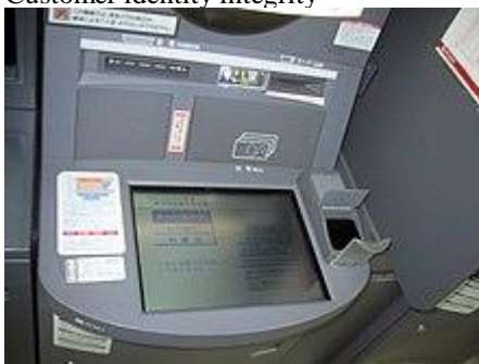
A BTMU ATM with a palm scanner (to the right of the screen)
