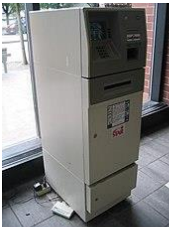
A Diebold 1063ix with a dial-up modem visible at the base
