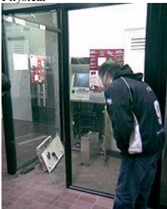
A Wincor Nixdorf Procash 2100xe Frontload that was opened with an angle grinder
