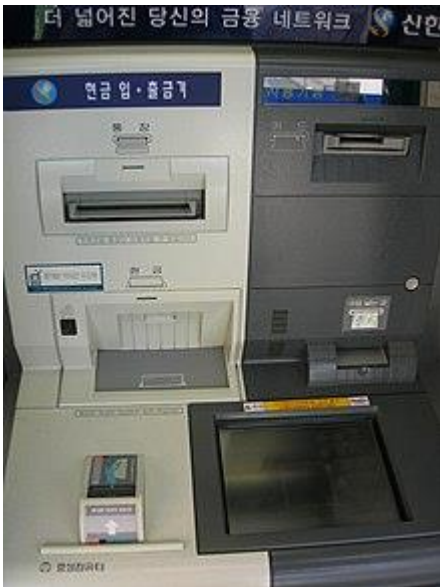
A South Korean ATM with mobile bank port and bar code reader
