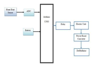
**Heartbeat sensor:** The heartbeat sensor comprises ECG electrode in which diagnoses the arrhythmia of the heart. For better extraction of the heart rhythm, the accelerated transducer is used. The heartbeat sensor is connected to the Arduino UNO board.
