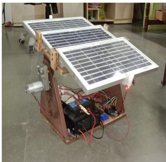
Fig.1. Solar tracking system.
