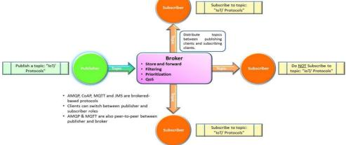
Figure 4 - Broker based architecture for data exchange
