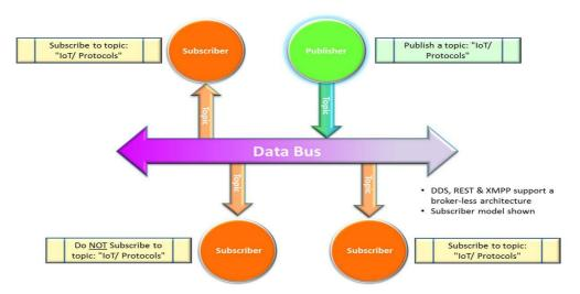
Figure 5– Bus based Architecture
