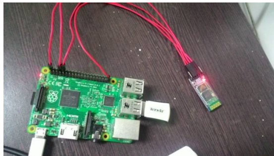
Figure 4. hardware interface between Raspberry Pi and Bluetooth
