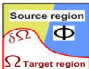
Fig.2: shows the input image with target region, source region and the boundary
