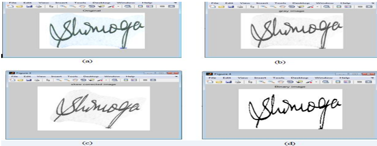
Fig.3 (a) Input image (b) gray scale (c) skew corrected (d) binary image
