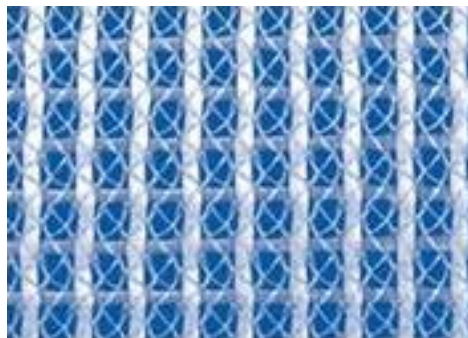
Figure 3. Illustration of a stitch-bonded fabric
