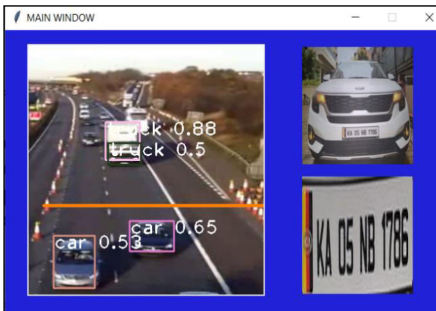
Fig. 3. Identification of vehicles through real time traffic video(left) Vehicle number plate detection and message notification (right)
