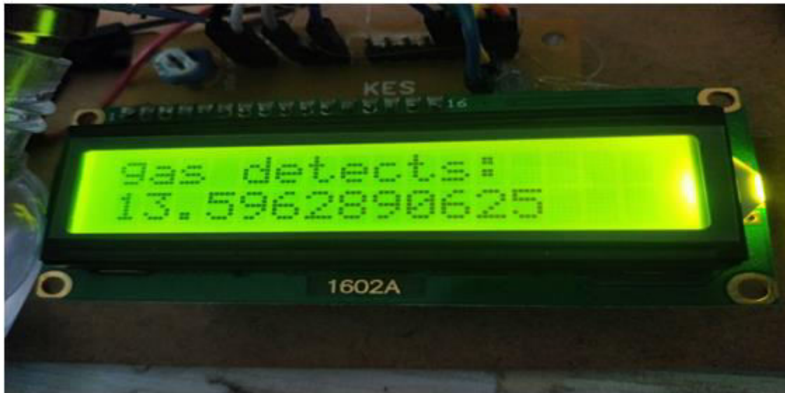
Fig.4.5 :MQ2 Sensor value shown in LCD
