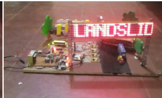
Fig. 9 Ultrasonic sensor detect landslide happened in hilly area
