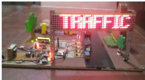
Fig. 10 IR Sensor detect traffic jam on the road
