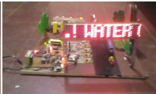
Fig. 7 Water Sensor detect water over the bridge
