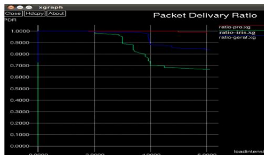
Fig 8b.Packet delivery ratio for ALBA-R versus GeRaF and IRIS.
