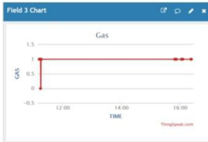
Fig 6. Webpage showing Gas Concentration around the miner
