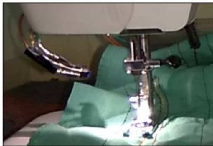
Fig 1: TCRT-5000 sensing the movement of needle in sewing machine
