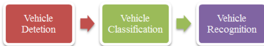
Figure 1: Illustrates the Block diagram that shows the three main stages of the ITS.
