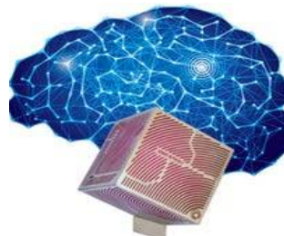
Fig.3: The EmoSpark console contains a 1.8 GHz CPU along with 2 GB of DDR3 memory and Rosenthal's custom-built 20 MHz EPU (Emotion Processing Unit)
