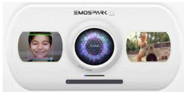
Fig.1: The EmoSpark uses facial recognition technology to interpret a user's expressions and develop a profile of his or her personality and emotional states.
