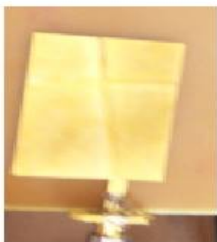
Fig.7 Photo of the fabricated Microstrip Antenna Fig.8 Simulated R. L. for proposed Microstrip Antenna
