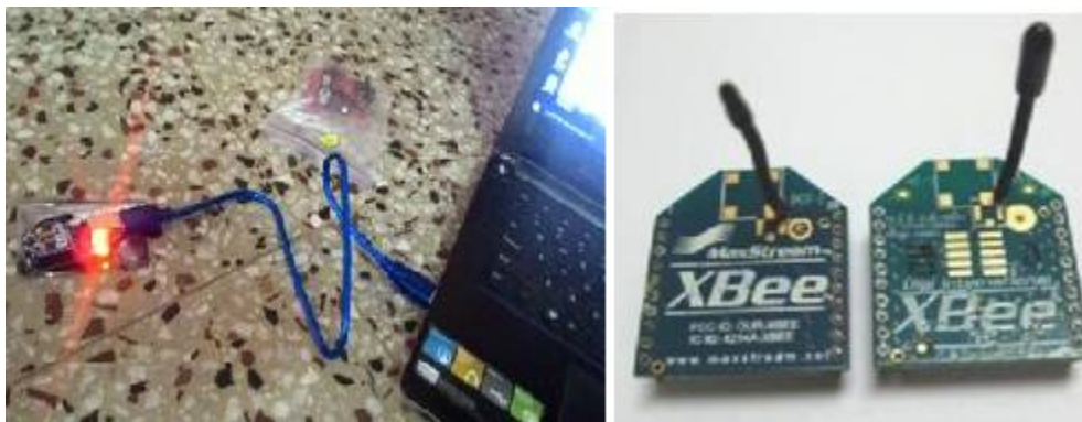
Fig. 2. Setup of Zigbee & Transmitter and receiver Zigbee for WSN
