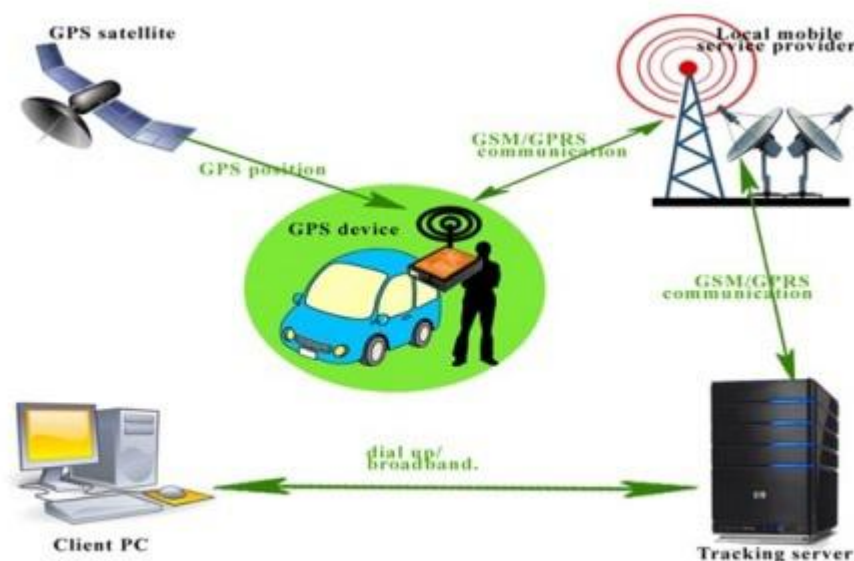
Fig1: Working of the GPS
