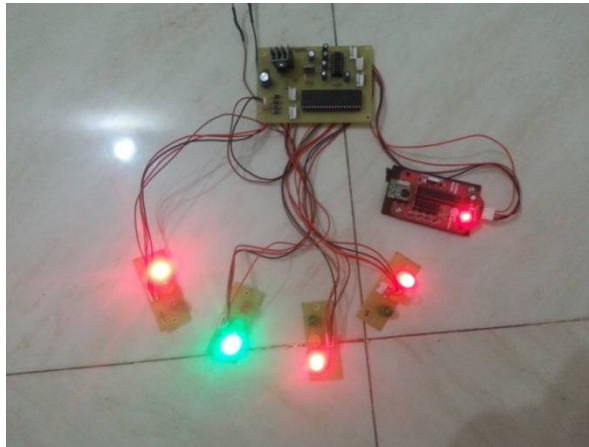
Fig 7. Traffic control unit displaying traffic signals
