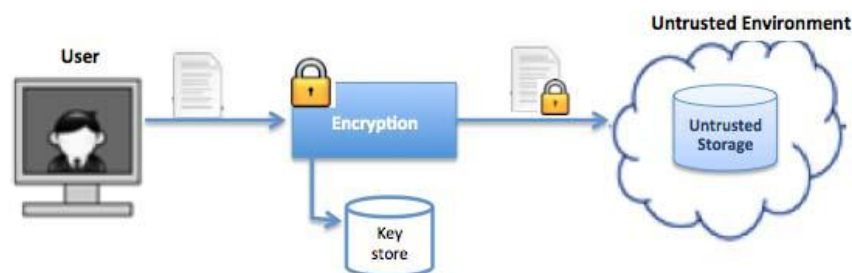
Fig 1: Architecture of secure data storage
