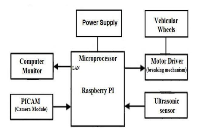
Traffic Sign Recognition: For the purpose of sign recognition the Raspberry Pi Camera is used. The Raspberry Pi Camera Board plugs directly into the CSI connector on the Raspberry Pi. It's able to deliver a crystal clear 5MP resolution image. This camera will capture images of traffic sign and send it to the raspberry pi controller board. Input image is then is analysed using machine learning algorithm which will able to detect the traffic sign.
