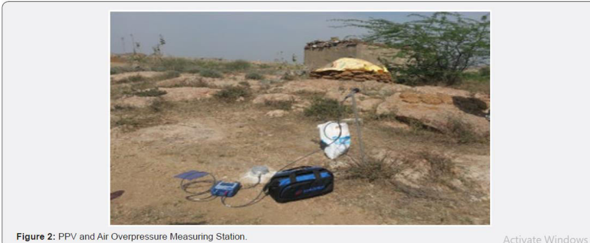
Figure 2: PPV and Air Overpressure Measuring Station.
