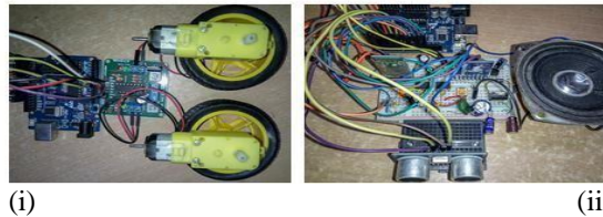
Fig. 3: Implemented model view of proposed robot (i) Motor driver circuit, (ii) Amplifier, Bluetooth and sonar sensor circuit
