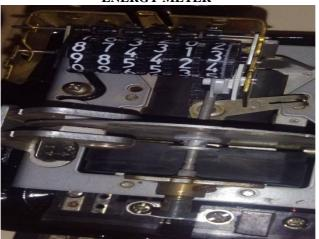
An energy meter could be a device that measures the number of electrical energy consumed by a residence or associate electrically battery-powered device. Electric utilities use electrical meters put in at customers' premises to live electrical energy delivered to their customers for request functions. They're generally label in request units, the foremost common one being the kW-hr [kWh]. They're typically scan once every request amount.
