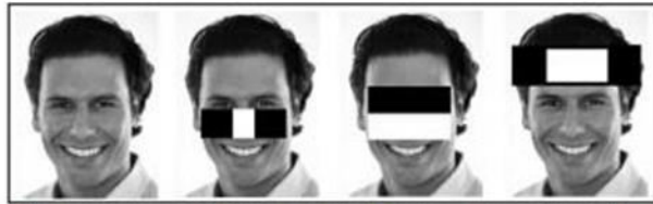
Figure 3: Examples of Haar features. Areas of white and black regions are multiplied by their respective weights and then summed up to get the Haar feature value.
