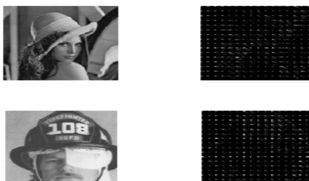
Figure 2: Original Image and Compressed Image with 8x8 DCT
