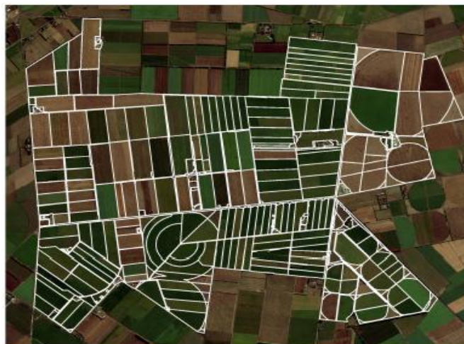
Figure 3: Hand-delineated reference fields, overlaid on the high-resolution satellite imagery from which they were derived (0.6 m pixel size).
