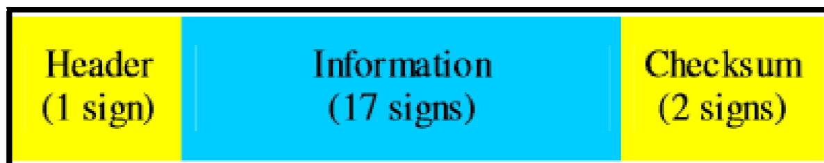
Fig. 2 Structure of watermark “word”
