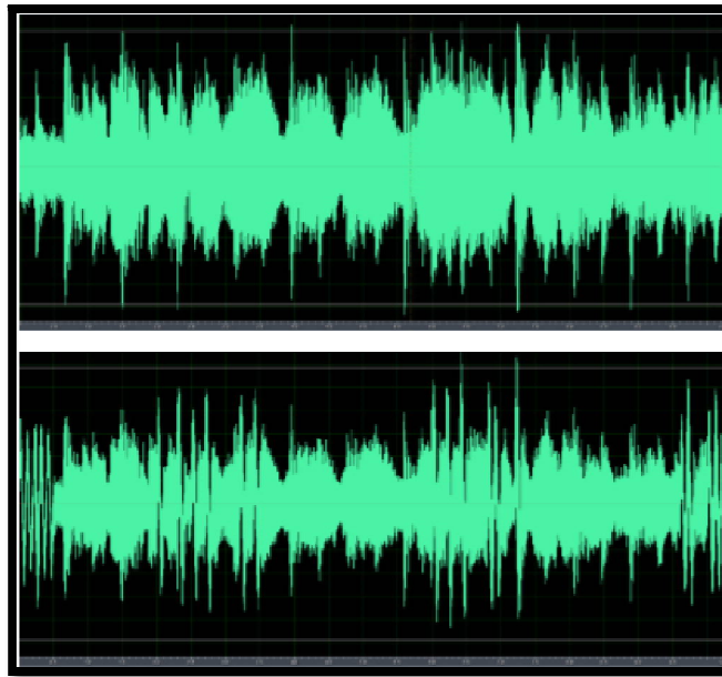
Fig.3 Comparison between original (top) and watermarked (bottom) audio files in time domain
