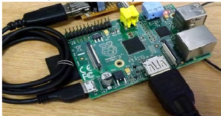
Fig.10. Raspberry pi connection with UART
