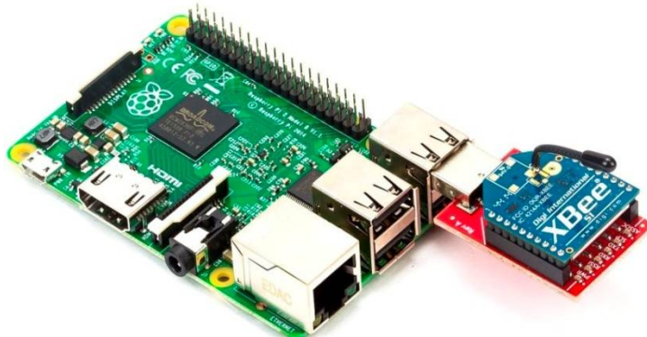
Fig.9. XBee is configured with Raspberry pi
