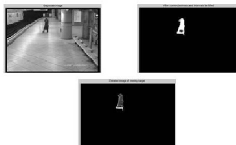
Figure. 5: Result for moving target detection algorithm based on dynamic background
