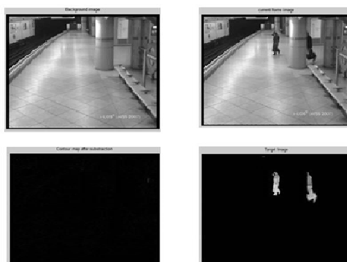
Figure. 2: Result of background subtraction Algorithm
