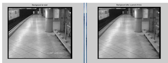
Figure. 3:Result of the background image at the different time
