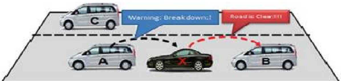
Fig. 5 Message alteration attack in V2V
