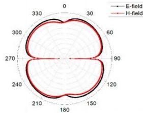
Figure 3. Radiation pattern for mode 1 at 5.8GHz
