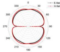
Figure 5. Radiation pattern for mode 3 at 5.8 GHz.
