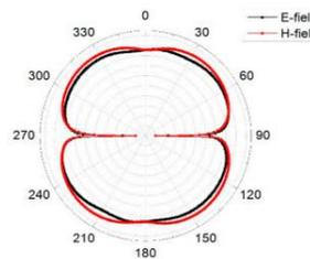
Figure 4. Radiation pattern for mode 2 at 5.8GHz
