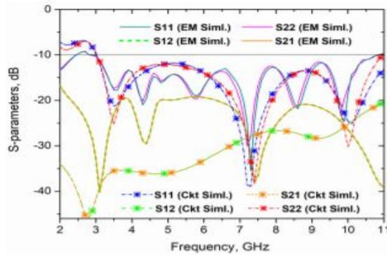
Figure 9. Equivalent circuit response and EM-simulated response of the proposed antenna.
