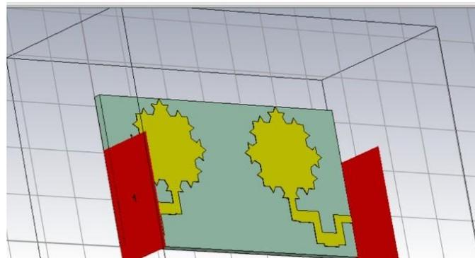
Figure 8. 3-D view of 2-port MIMO antenna
