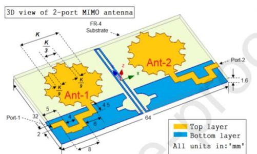
Figure 6. Geometry of the proposed 2-port MIMO antenna.
