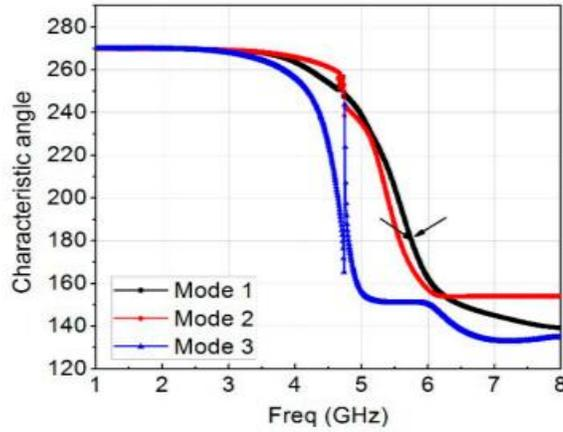
Figure 2. Characteristic angle of three modes at 5.8 GHz
