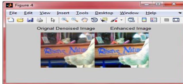
Figure 1.12: Window with Denoised fused image and Enhanced image using DWT-2 nd Level
