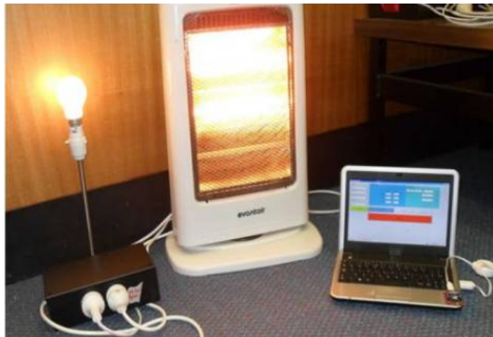
Fig.3. Smart power monitoring and control system at the residence.
