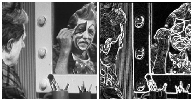
Figure 3: Edge detection of a clown image with the Sobel operator
