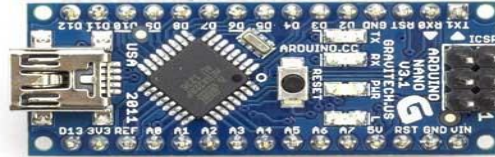
Figure 4. Hardware Architecture of Arduino NANO
