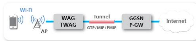
Fig1: Trusted 3GPP Wi-Fi access
